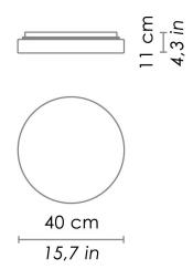
Wall-ceiling lamps with diffuser in mouth-blown, satin-finish opal triplex glass; chlorine-resistant, anti-UV, neutral translucent polycarbonate frame. Twist-lock coupling system for the glass component. The product is suitable for indoor use only. The Drum collection is IP44.
